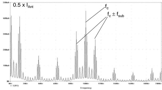
**Figure 17** shows the frequency spectrum of the output signal of the ASK modulator with an endless sequence of 1-bits.
