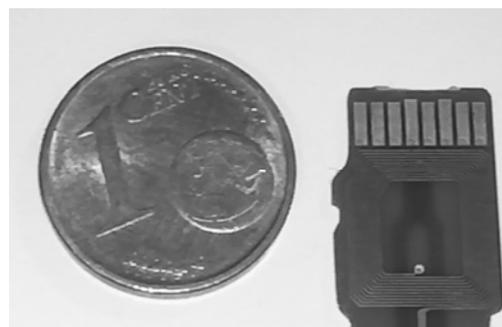
**Figure 8:** Size comparison –micro-SD sized transponder antenna
