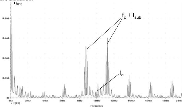
**Figure 15** shows the frequency spectrum of the output signal of an optimized ring modulator with an endless sequence of 1-bits. The carrier frequency  $f_c$  (13.56 MHz) is clearly suppressed.
